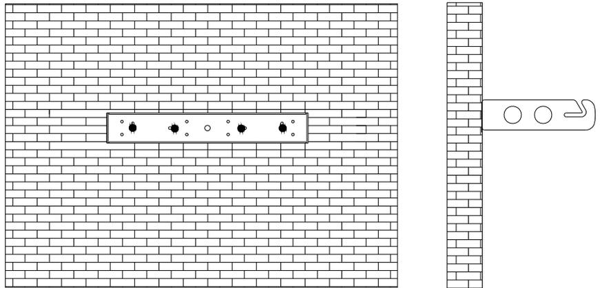
*Drill some corresponding pilot holes on the wall and fix the bracket with some screws.*
