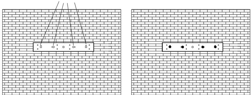
*Place the SP-8 bracket in front of the mounting surface, so you can mark the locations of the mounting holes.*
